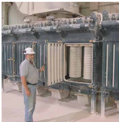
Louvered door inlet for cross-flow applications
